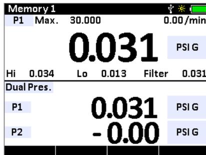
To test a sensor without an electrical output, set the HPC40 Series to a pressure only screen with an accuracy of 0.035% of reading.
