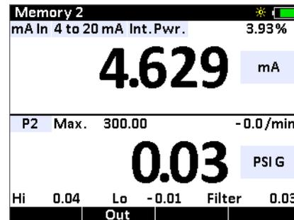
To test a transducer with an electrical output, set the HPC40 Series upper window to measure mA, and the lower window to measure pressure.
