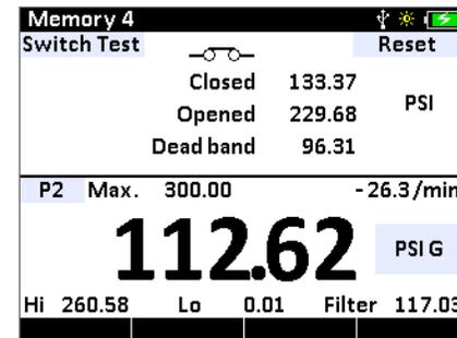
To test a switch, the HPC40 Series has a dedicated screen that will display the open, close, and dead band values of the switch. The lower screen will always show the live pressure.
