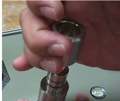
*Grasp the nozzle firmly and pull upward with a slight twisting motion.*
