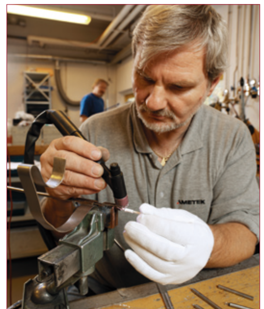
Welding of mineral insulated RTD's
