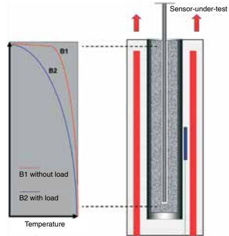
The temperature gradient, and consequently the uncertainty in the calibration process becomes unmanageable. A similar gradient also applies to other short sensors that do not reach the bottom of the calibration block.
