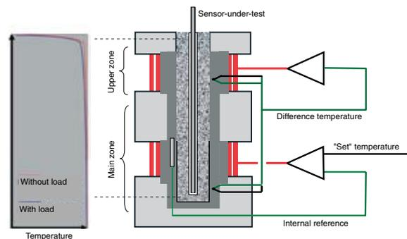
The illustration above shows the dual-zone design. The graph indicates how the temperature is kept uniform despite the load.
