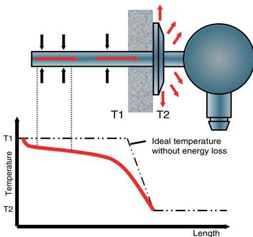
The figure above graphically illustrates a temperature measurement through an isolating wall. The sensor is a Pt100 element with a specific extension meaning that the sensor will measure an average of its own temperature and the process temperature. It is obvious that there is a temperature gradient along the entire length of the sensor; this is indicative of the energy loss to ambient conditions.
